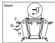
Screw down Bolt(I) as shown, Then Attach Legs(H) and Middle Leg (K) to the bottom with Bolt (G) and Allen key (J) as picture shows.
