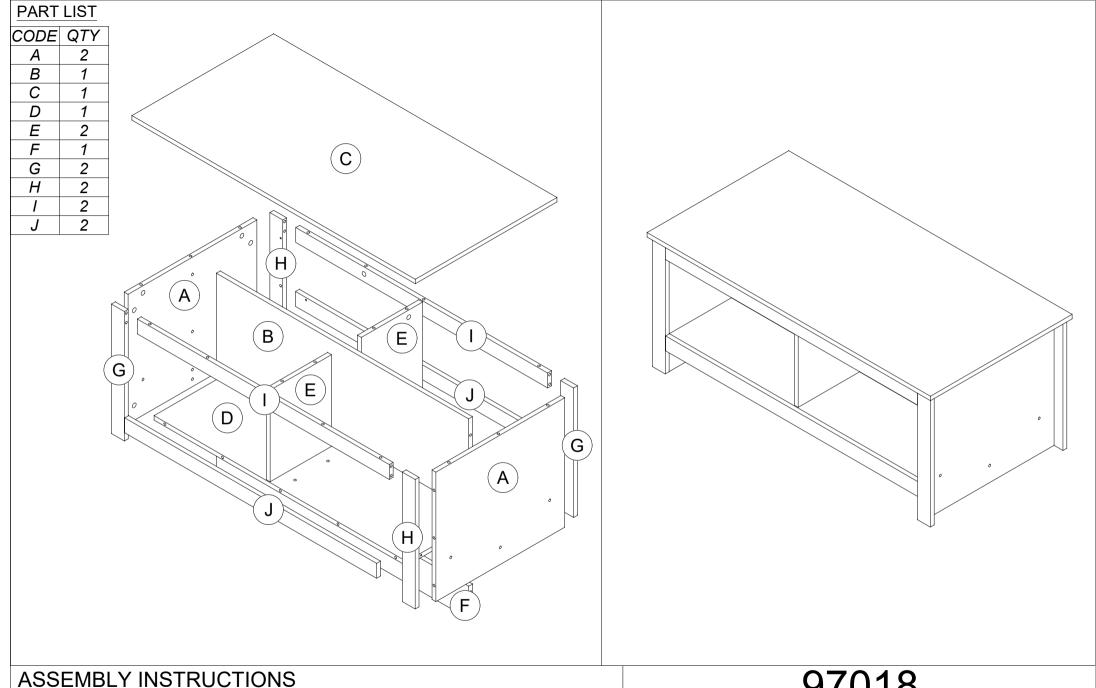
DO NOT FULLY TIGHTEN ANY BOLTS BEFORE ALL PARTS ARE LOOSELY ASSEMBLED. THE PRODUCT/FITTINGS MAY BE DAMAGED IF OVERTIGHTENED. BEWARE OF CROSS THREADING SCREWS AND BOLTS DURINGS ASSEMBLY. SMALL COMPONENT PARTS COULD CHOKE A CHILD IF SWALLOWED. WE STRONGLY RECOMMEND THAT YOU KEEP CHILDREN AWAY FROM THE WORK AREA.
